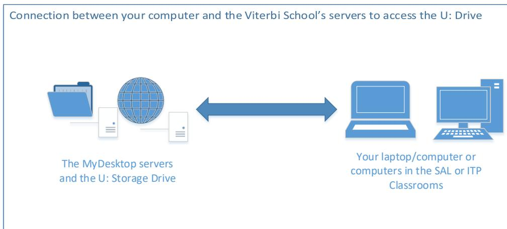
Here is a diagram of how MyDesktop and your computing device work in tandem. When working on an assignment, the files are accessed by the Viterbi School's servers in real time. The servers supporting MyDesktop are connected directly to the U: Storage Drive. This direct connection reduces latency between MyDesktop and the Storage Drives. This method would be faster than connecting a USB flash drive on your computer and sharing that with MyDesktop.
